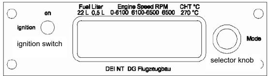
After turning on the main switch the DEI-NT shows a screen with operating times.
